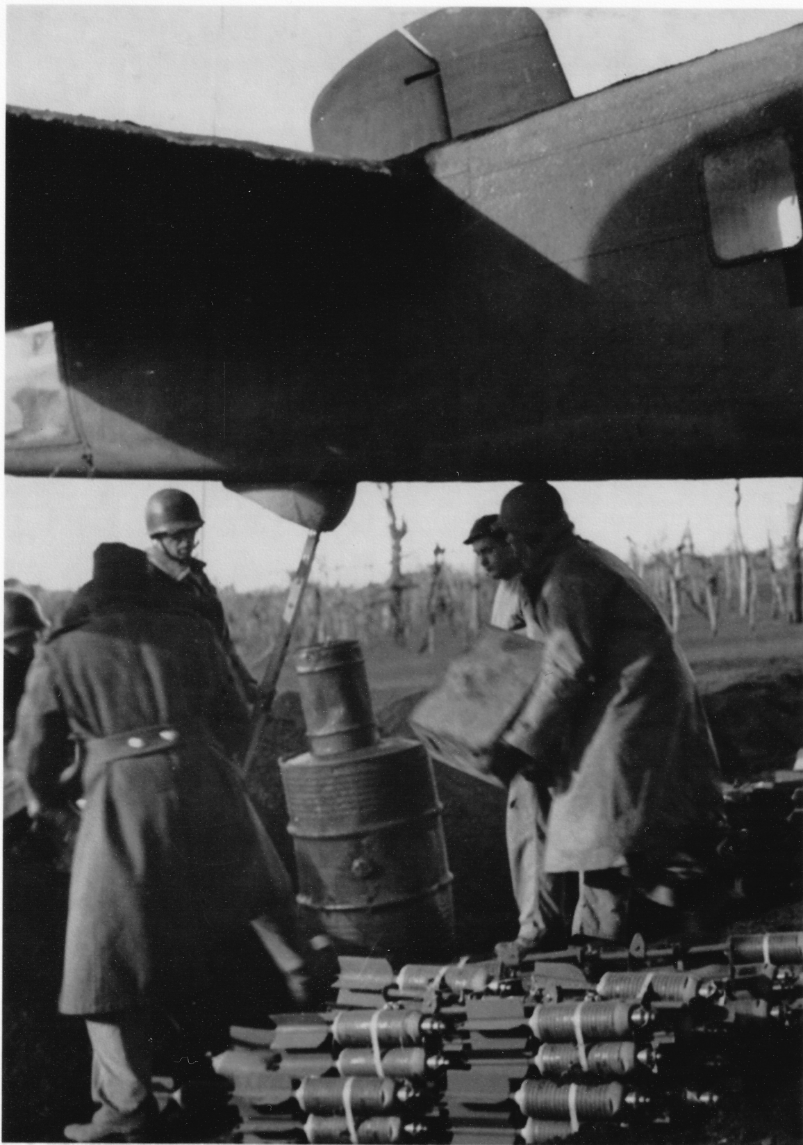
Men of the 340th Bomb Group jack up the tail of a North American B-25 which was damaged during the eruption of Mt. Vesuvius on 23 March 1944. Note fragmentation bombs uncovered and cleaned off.
